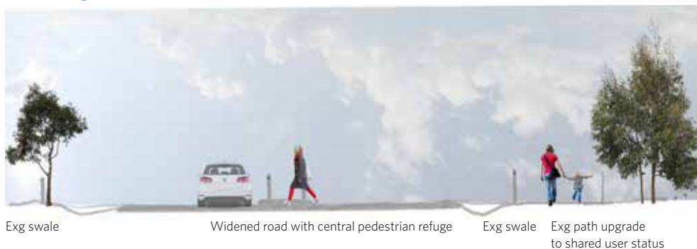
Figure 6: Possible Pedestrian Facilities
