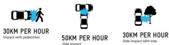
Figure 5. Survivable impact speeds for different crash types.
